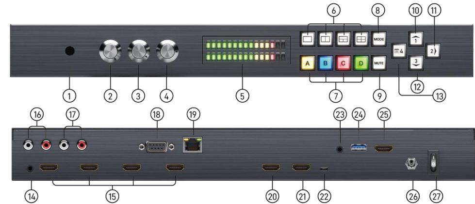
1. **IR SENSOR:** IR sensor for receiving the IR commands from IR remote
